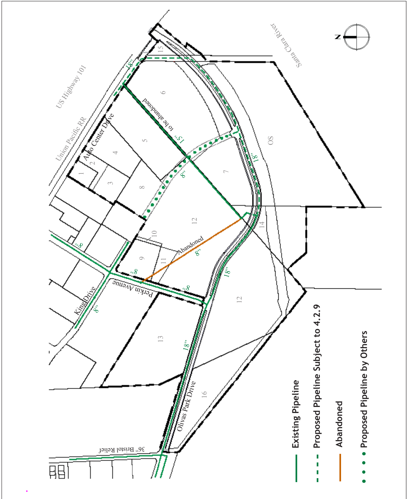
FIGURE 4-4 PROPOSED BACKBONE WASTEWATER SYSTEM
